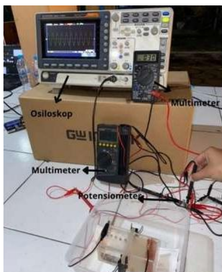
Figure 3. Set up MFCs to measure Power, Voltage, and Current Using Potentiometer on MFCs
