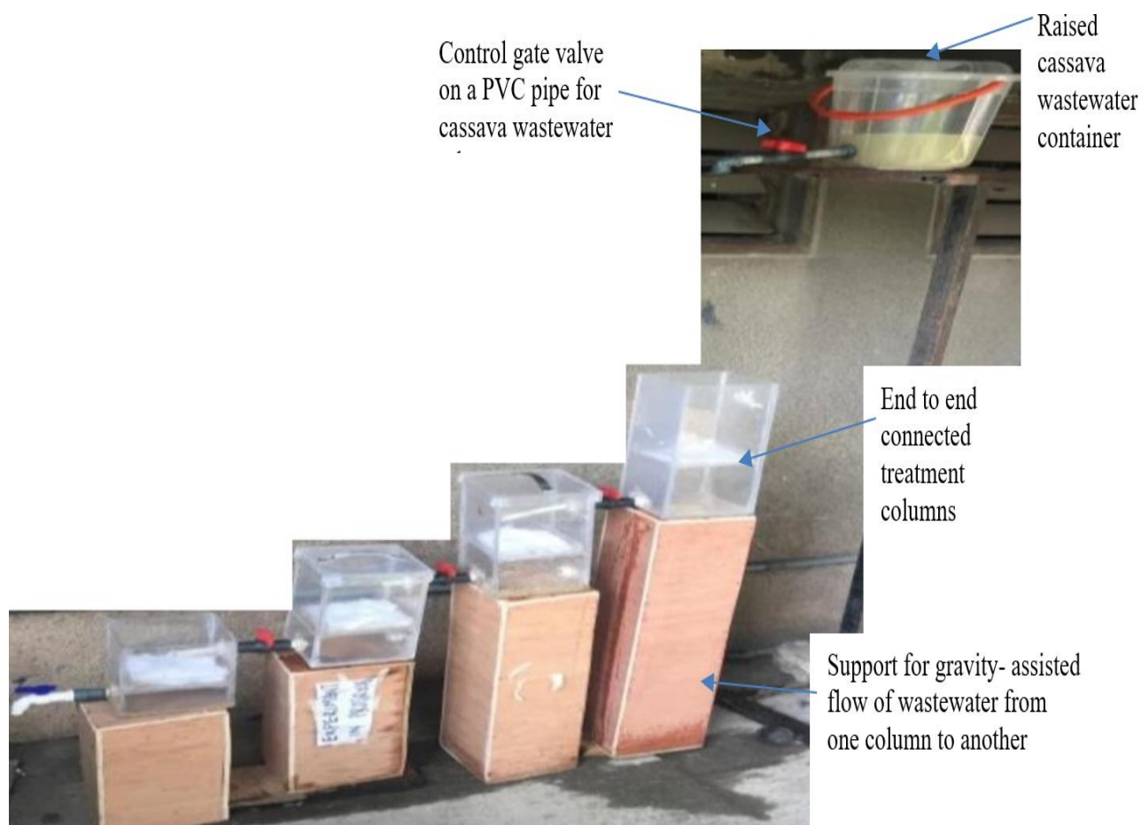
Figure 2. The Cassava Wastewater Treatment System without Recirculation (CWTS-WR) under loading conditions
