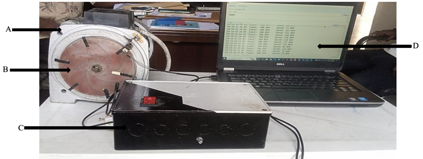
Figure 11. Complete setup of the SyncRM drive system
