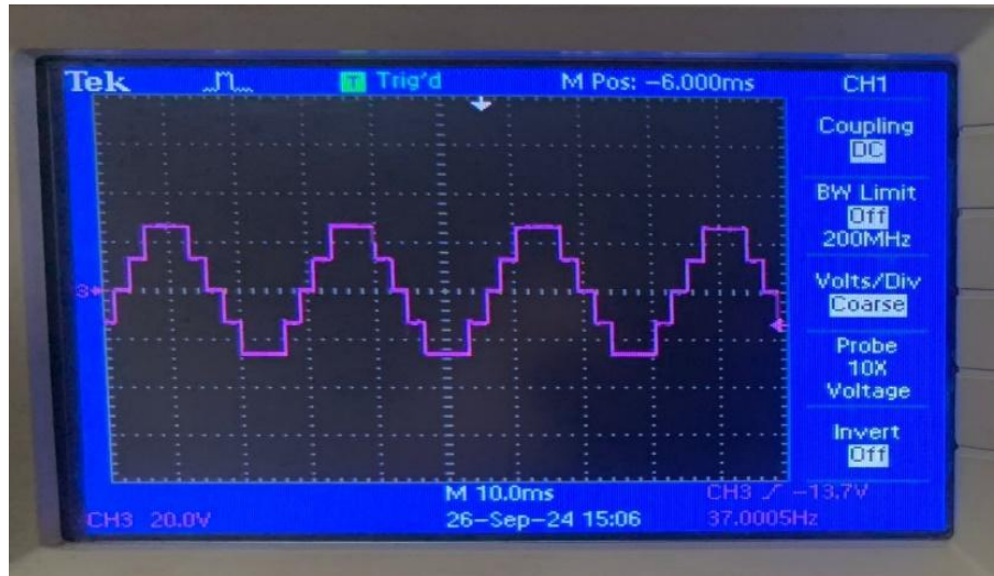
Figure 8. Experimental Voltage Output Waveform of the 5-Level CHB Inverter
