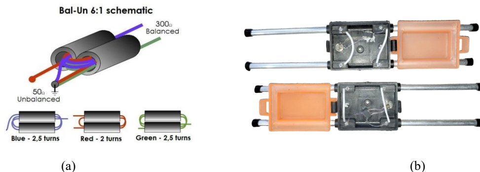
Figure 2. Components of the Yagi Antenna (a) Design Planning, b) Yagi Antenna design results on Dipole
