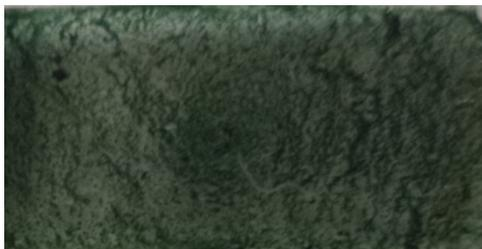
**Gambar 1.** Hasil spin coating lapisan tipis PANi/PVA diatas ITO
