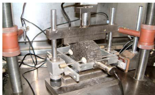
Gambar 1. Indirect Tensile Stiffness Modulus (ITSM) test
