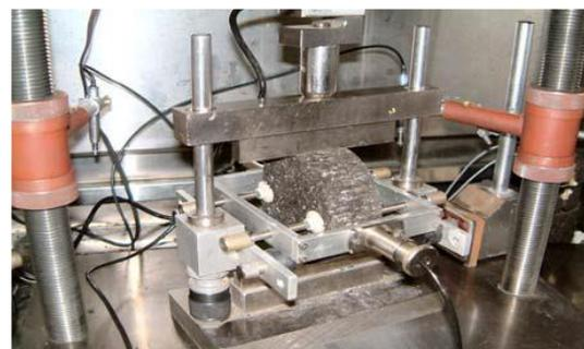
Gambar 1. *Indirect Tensile Stiffness Modulus (ITSM) test*
