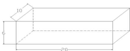
Gambar 1. Dimensi paving block
