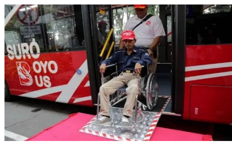
Figure 2. Disabled facilities in the form of wheelchair ramps. Source: Surabaya Transportation Department
