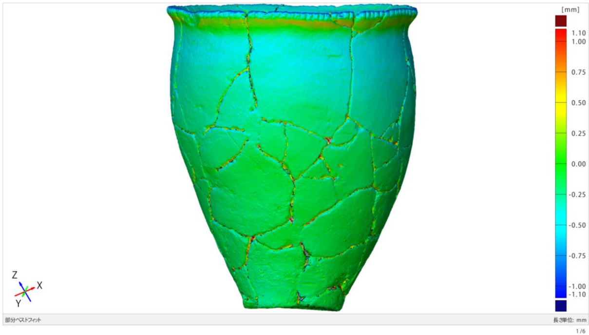
Fig.4. Compared results of the jar with GOM Inspect. This figure show that smaller differences is green color and bigger differences is red color. This material has bigger differences on its tip and crack. The jar of Ongagawa style in Tamura sute is stored by Kochi Prefecture Board of Education.
