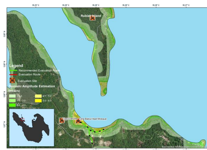
Figure 10. Iboih Inundation Map. Recommendations of evacuation routes and sites based on the numerical tsunami simulation (green line)
