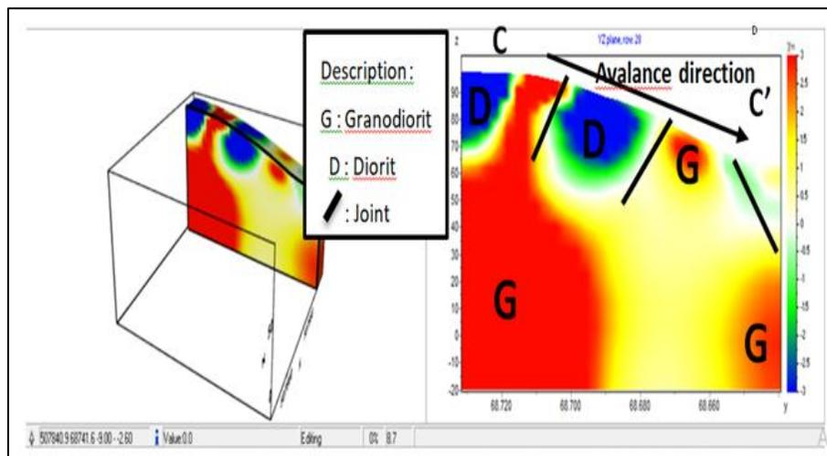
**Figure 12.** 2D and 3D Modeling (Section C – C')
