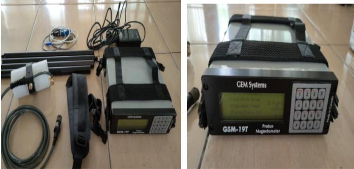
**Figure 1.** Proton Precession Magnetometer GSM-19T
