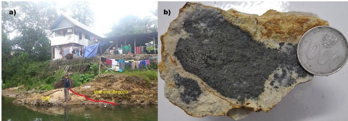
Figure 2. (a) Volcanic breccia and tuff outcrops found near the ERT line, (b) Close up view of tuff
