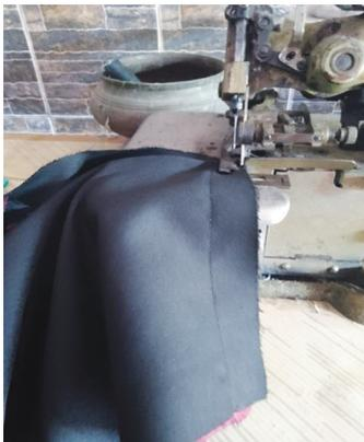
**Gambar 13 Mengobras Bagian Bahu**
