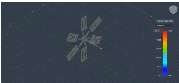
Fig. 10. Sink Mark Defect (Medium)
