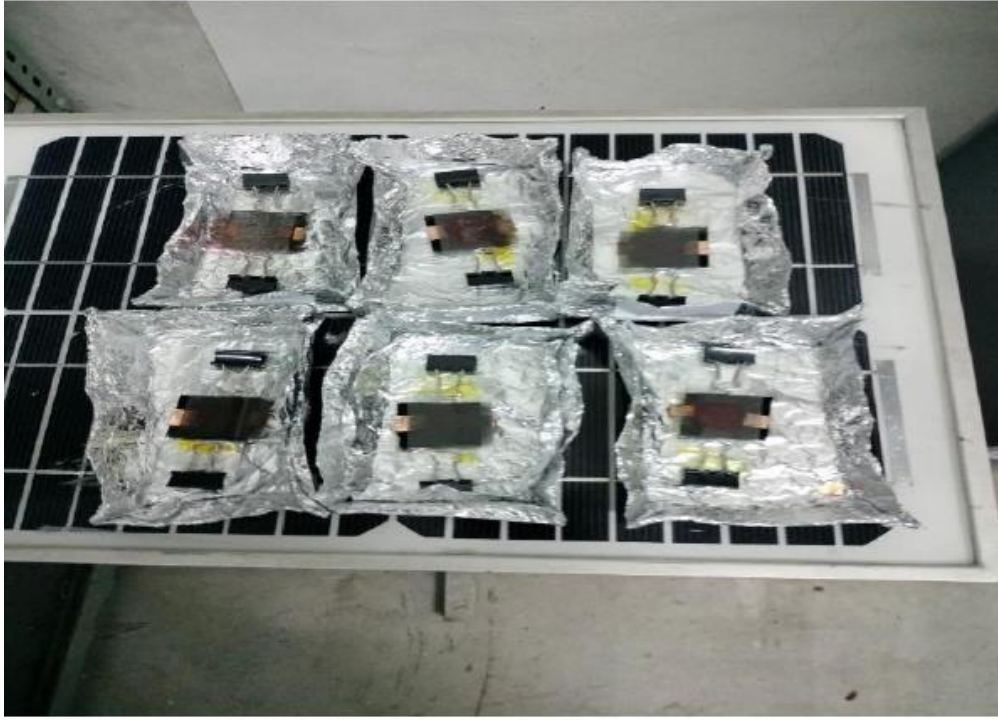
Figure 1. Original graphite:PVA-DMSO film samples S1-S6.
