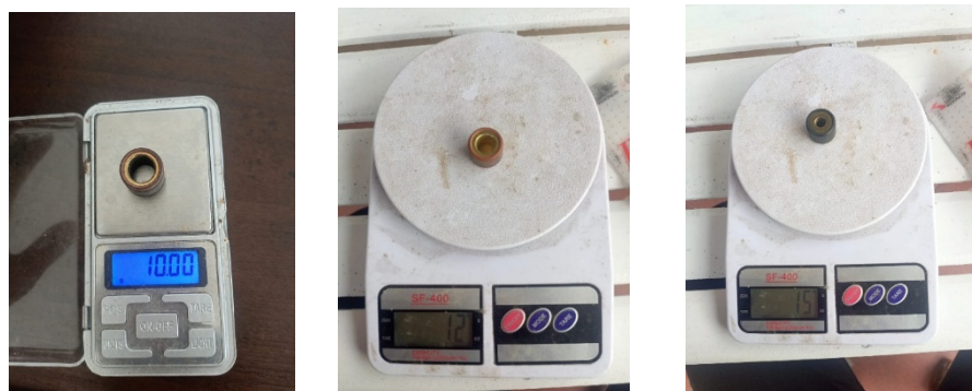
Figure 2. Roller weight 10 grams, 12 grams, 15 grams
