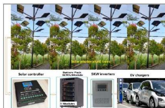
Figure 3. Schematic solar photovoltaic for electric vehicle charger
