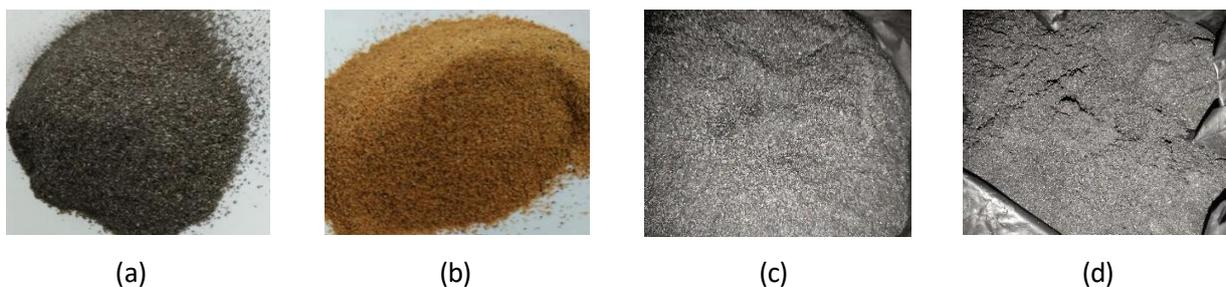
**Figure 1.** Recycled aluminium powder (a), Silica sand (b), Rice husk ash (c), Bagasse ash (d)
