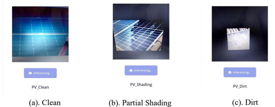
**Figure 8.** Model inference test in recognizing clean (PV\_Clean), dirty (PV\_Dirt) and shading (PV\_Shading) cells.
