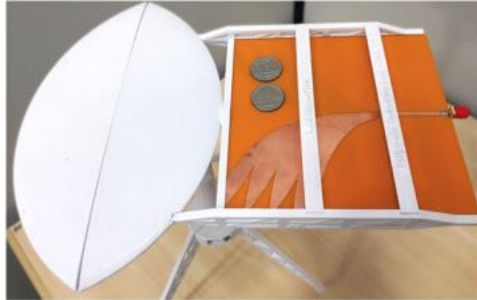
Figure 7. Depicts a Palm Tree class AVA with a PLA filament lens [15].
