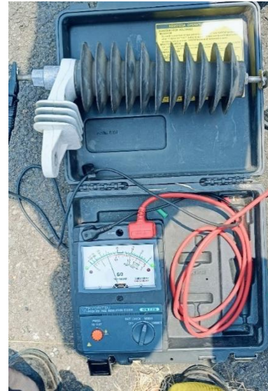
Figure 3. Lightning Arrester isolation detention measurement
