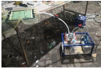
Figure 9. Vacuum Infusion Process of FML Specimen (Source: Author's own documentation)
