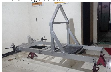
Figure 5. Chassis made from Hollow Aluminum Alloy
