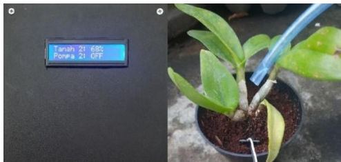
Figure 14. Testing Soil Moisture Sensor and Water Pump on Coconut Fibre Planting Media
