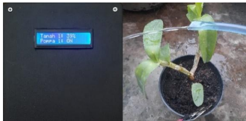
Figure 13. Testing Soil Moisture Sensor and Water Pump on Fertiliser Kascing Planting Media
