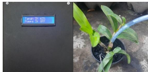
Figure 15. Testing Soil Moisture Sensor and Water Pump on Charcoal Planting Media
