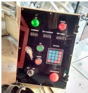
Gambar 6 Elektrical Control Unit (ECU)
