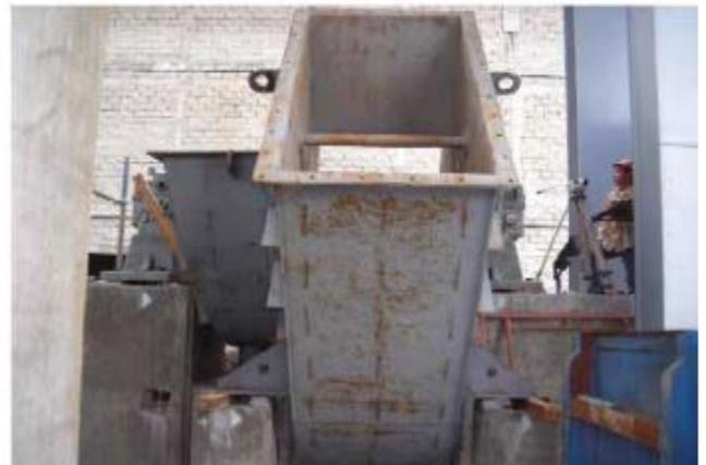
Gambar 5 Casing PA Fan
