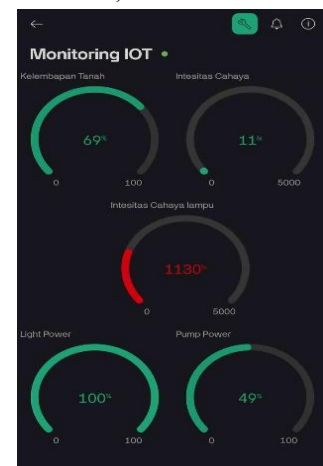
Figure 8. Real-Time Monitoring Interface via Blynk Platform
