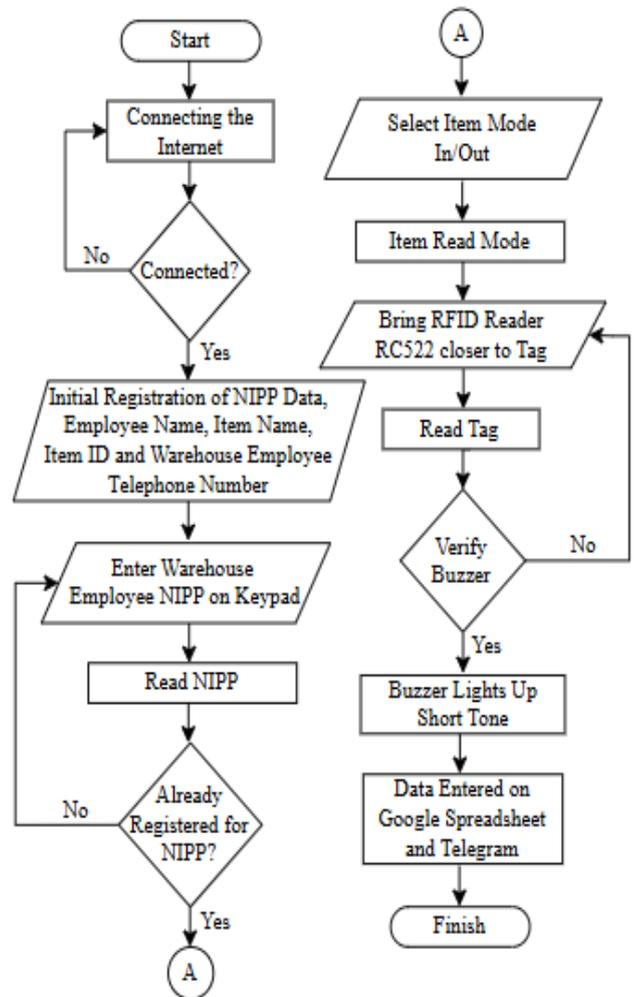
Figure 4. Flowchart designing software
