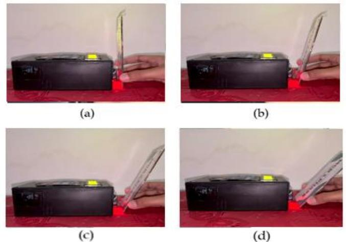
**Gambar 6.** RFID Label sticker testing with various positions, (a) 0° (b) 15° (c) 30° (d) 45°
