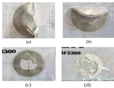
**Figure 9.** Physical condition of RFID label stickers, (a) vertically folded (b) horizontally folded (c) good condition (d) wet
