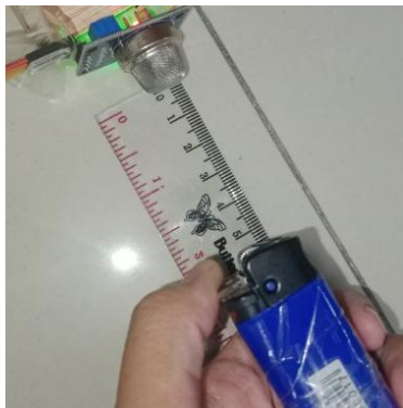
Figure 15. Illustration of MQ-6 Sensor Testing in an Open Space
