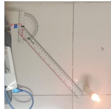
Figure 12. Illustration of KY-026 sensor detection accuracy test
