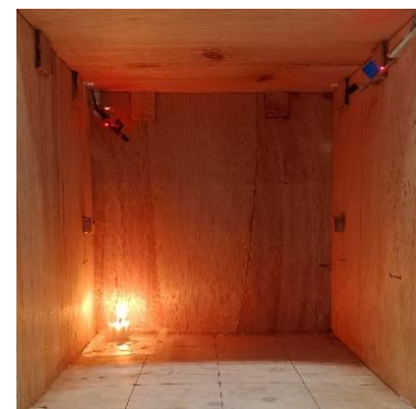
Figure 13. Blind Spot Testing Illustration from Using Two KY-026 Sensors
