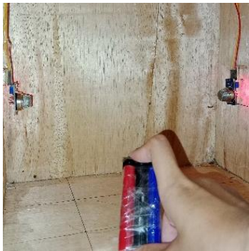
Figure 18. Illustration of Response Time Testing of Two MQ-6 Sensors
