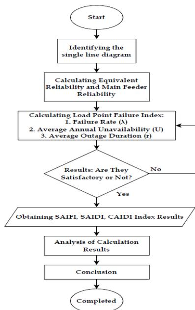
Figure 4. Block Diagram of the RNEA Method Calculation
