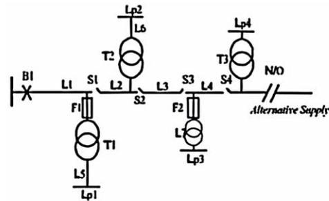
Figure 1. Radial Distribution System
