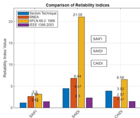
Figure 6. Evaluation Graph of Reliability Indices Using SPLN 68-2:1986 and IEEE 1366-2003
