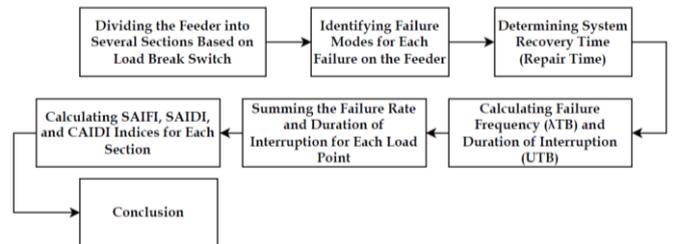
Figure 3. Calculation Flowchart for the Section Technique Method
