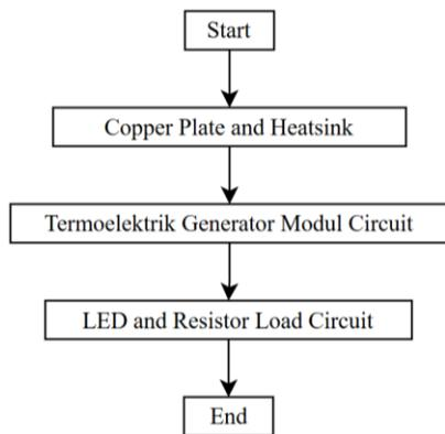
Figure 4. STEG block diagram system
