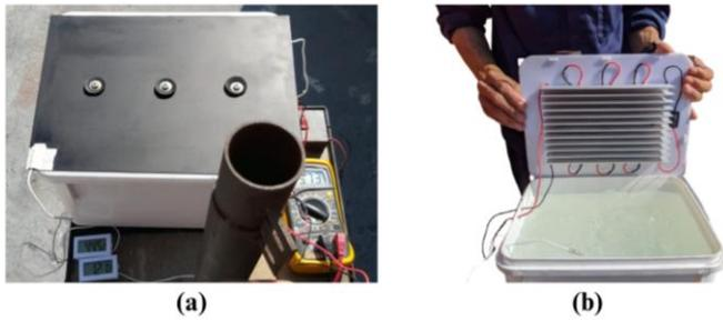
Figure 6. STEG Prototype assembly result (a) view from above STEG (b) inside view from STEG
