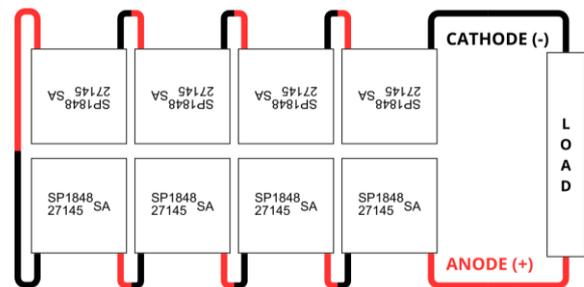
Figure 2. STEG and load circuit configuration
