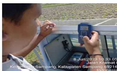
Figure 7. The process of taking solar radiation data
