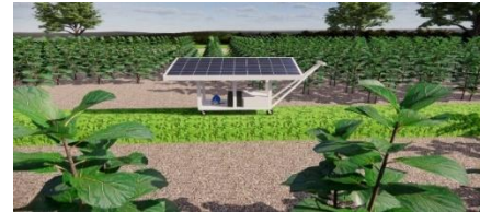
Figure 3. Design of 3D Portable Solar Water Pump
