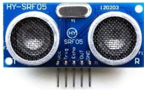
Figure 2.2. SRF05 Ultrasonic Sensor
