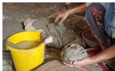
Figure 7. Clay being kneaded before the process of shaping the cowek
