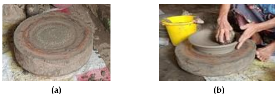
Figure 3. (a) The perbot tool; (b) The cowek formatting process
