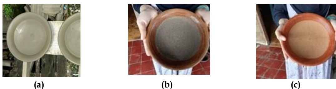
Figure 10. (a) The Process of a cowek when aired; (b) The look of the cowek ready to be burned; (c) The look of the cowek after being burned
