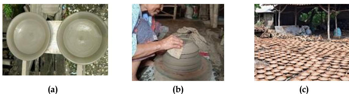
Figure 4. (a) Drying process; (b) Ndalimi process (smoothing) after adding feet the bottom of cowek ; (c) Drying process after being colored red with red soil until completely dry.
