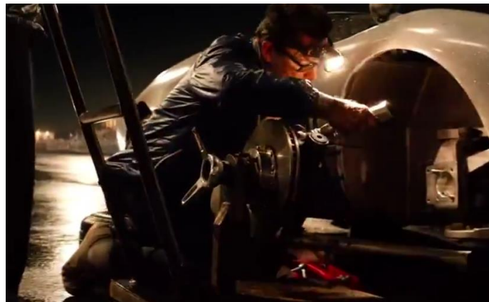
Figure 4. The Quick-Change Brake Assembly System Ford Employed in Their Second Le Mans Entry As Depicted In The Movie
