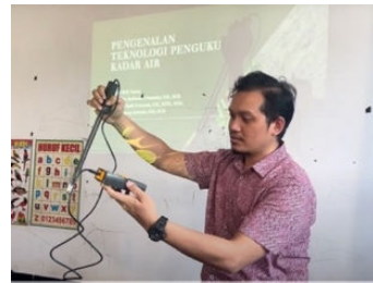
Gambar 4. Peragaan alat pengukur kelembapan simplisia
